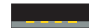
Road marking indicating prohibition to park. The marking is placed at the edge of the carriageway.
